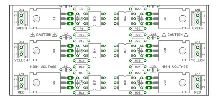
Insert the neutral wire (white) from your GREEN light into terminal "1" of CN5 and insert the hot wire (green) from your GREEN light into terminal "2" of CN5.
