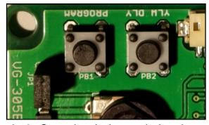
Green from left to right three (3) times to indicate mode 3. Once the desire mode has been selected, you can replace JP1 to exit the program mode.
